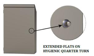
We first had to modify our hygienic quarter turn by adding extended flats so that a standard crescent wrench or open-ended box wrench could be used. We then redesigned the doors so one hygienic quarter turn with a 3-point cam and its interlocking rod assembly would be able to keep the door sealed properly.
